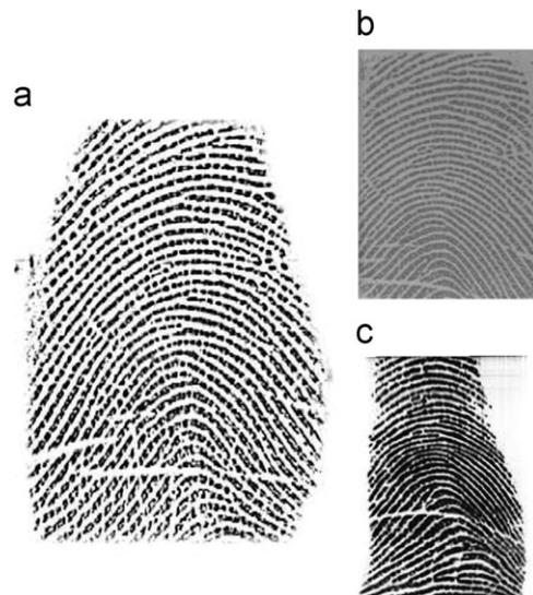
**Fig. 6.** Fingerprint samples of the same user of the FINGERPASS cross-matching database. (a) URU4000B; (b) UPEK TCRU2C; and (c) AES2501.
