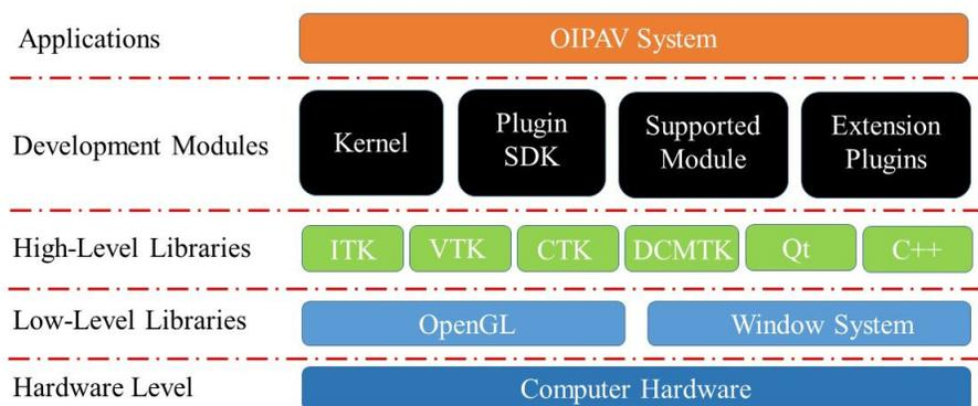
Fig. 1 General architecture of the system.
